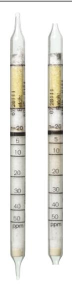
Standard Measuring Range: 5 to 50 ppmNumber of Strokes (n): 20Time for Measurement: app. 8 minStandard Deviation: ± 15 to 20 %Colour Change: pale gray →> orange
