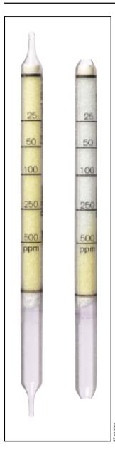
Standard Measuring Range : 25 to 500 ppm Number of Strokes (n) : 30 Time for Measurement Standard Deviation : app. 6 min : ± 20 to 30 % Colour Change : pale yellow —> turquoise green
