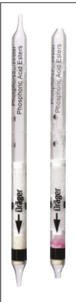
Standard Measuring Range : 0.05 ppm Dichlorvos
