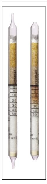
Standard Measuring Range : 20 to 250 ppm /2 to 50 ppm Number of Strokes (n)
