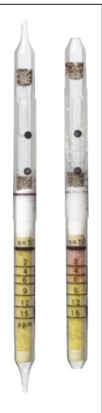
Standard Measuring Range : 2 to 15 mg/m<sup>3</sup>
