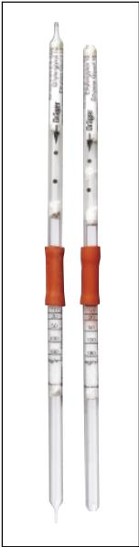
Standard Measuring Range: 10 to 180 mg/m<sup>3</sup>
