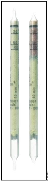
Standard Measuring Range : 20 to 100 mg H<sub>o</sub>O/m<sup>3</sup>
