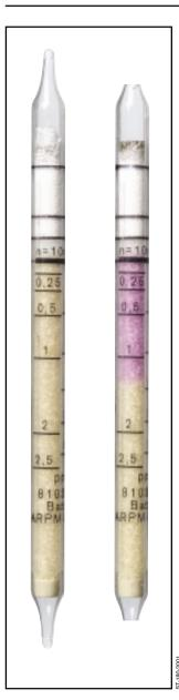
Standard Measuring Range : 0.1 to 2.5 ppm / 3 to 15 ppm Number of Strokes (n) : 10
