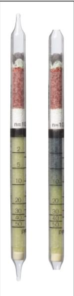
**Standard Measuring Range**: 5 to 100 ppm / 2 to 50 ppm
