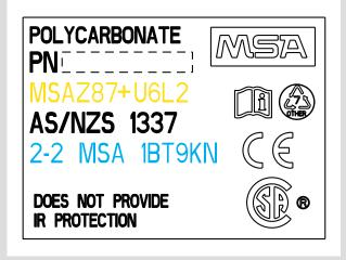
First marking line (in yellow) shows the visor is impact-rated to ANSI/ISEA Z87.1-2010 (Z87+), offers maximum UV filter (U6) as indicated under the Standard, and has a visible light transmission filter not more than 43% (i.e., it's tinted).
