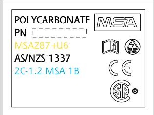
First marking line (in yellow) shows the visor is impact-rated to ANSI/ISEA Z87.1-2010 (Z87+), and offers maximum UV filter (U6) as indicated under the standard.
