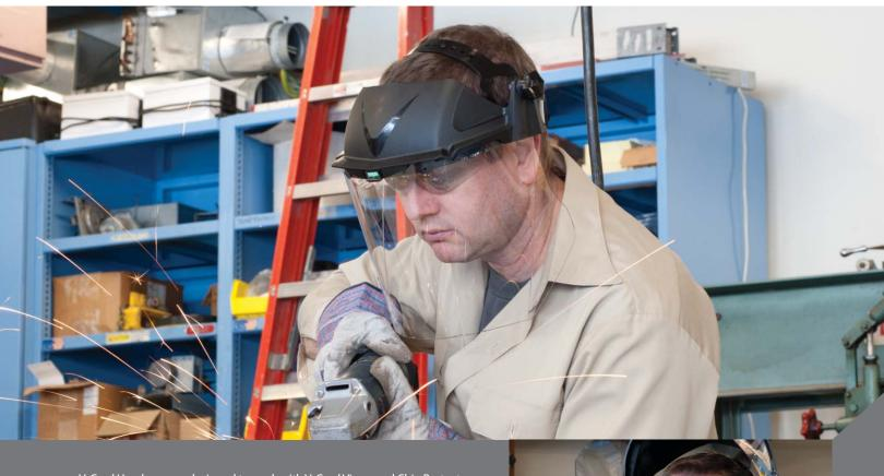
V-Gard Headgear are designed to work with V-Gard Visors and Chin Protectors, and meet many global standards, including ANSI/ISEA Z87.1-2010, CSA Z94.3, EN166 and AS/NZS 1337.
